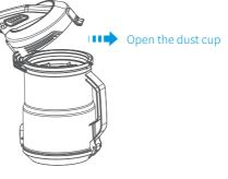
**02.** Remove the filter cotton for cleaning: Open the dust cup, remove the filter cotton and clean it.
