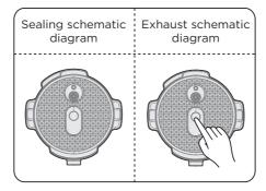
• Check if the floater valve drops down before working (before heating, the floater valve is down).
