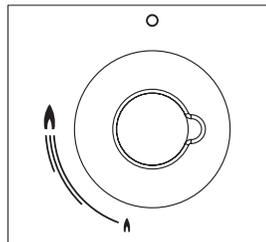
The small flame indicates the 'low position'. Turn the knob to it after the contents of a pan have boiled.
