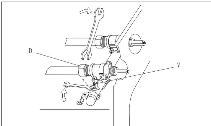
Clean the cone and it's slot by means of a cloth soaked with solvent.
