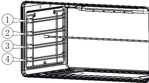
The accessories can be inserted in the oven in 4 different shelf positions. You can pull the accessories two-thirds of the way out without them tipping.
