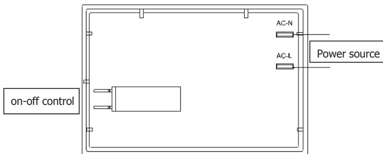
As shown in the picture, on-off control is used to control heating components of oven, the left is power source which can be connected under the 220V.
