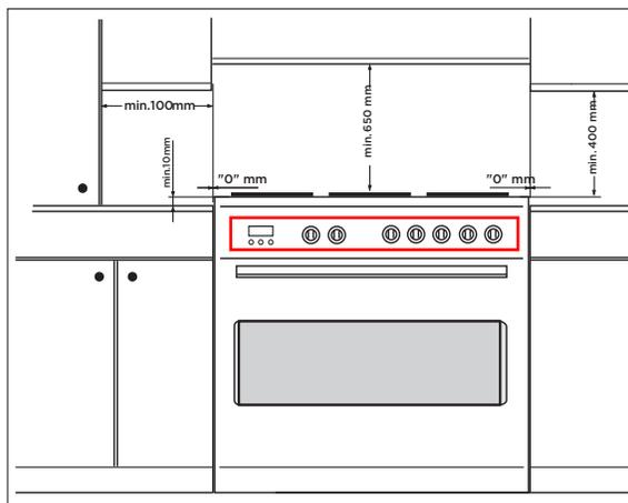
No part of any adjoining wall surface can be made of combustible materials. The protection of combustible materials required by Clause 5.12.1.1 of AS/NZS 5601 is the fixing of 5 mm thick ceramic tiles to the surface or attaching fire resistant material to the surface and covering with sheet metal with a minimum thickness of 0.4 mm.
