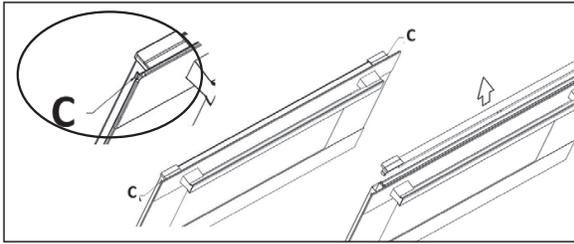
**▲ The inner glass of the oven with fixing snap (only for the models where is provided)**
