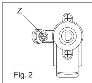
Unscrew the adjusting screw in order to increase the flow or screw it to decrease the flow.
