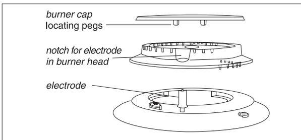
For a triple crown burner, make sure head “C” and covers “A” and “B” are properly placed on their seats as figure E and not off-centered as in figure F
