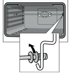
2. Carefully withdraw the rotary spit from the recessed adapter in the side panel and remove it from the oven.
