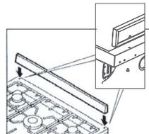
**▲ Fix the oven to the rear wall using the chain and screws supplied.**
