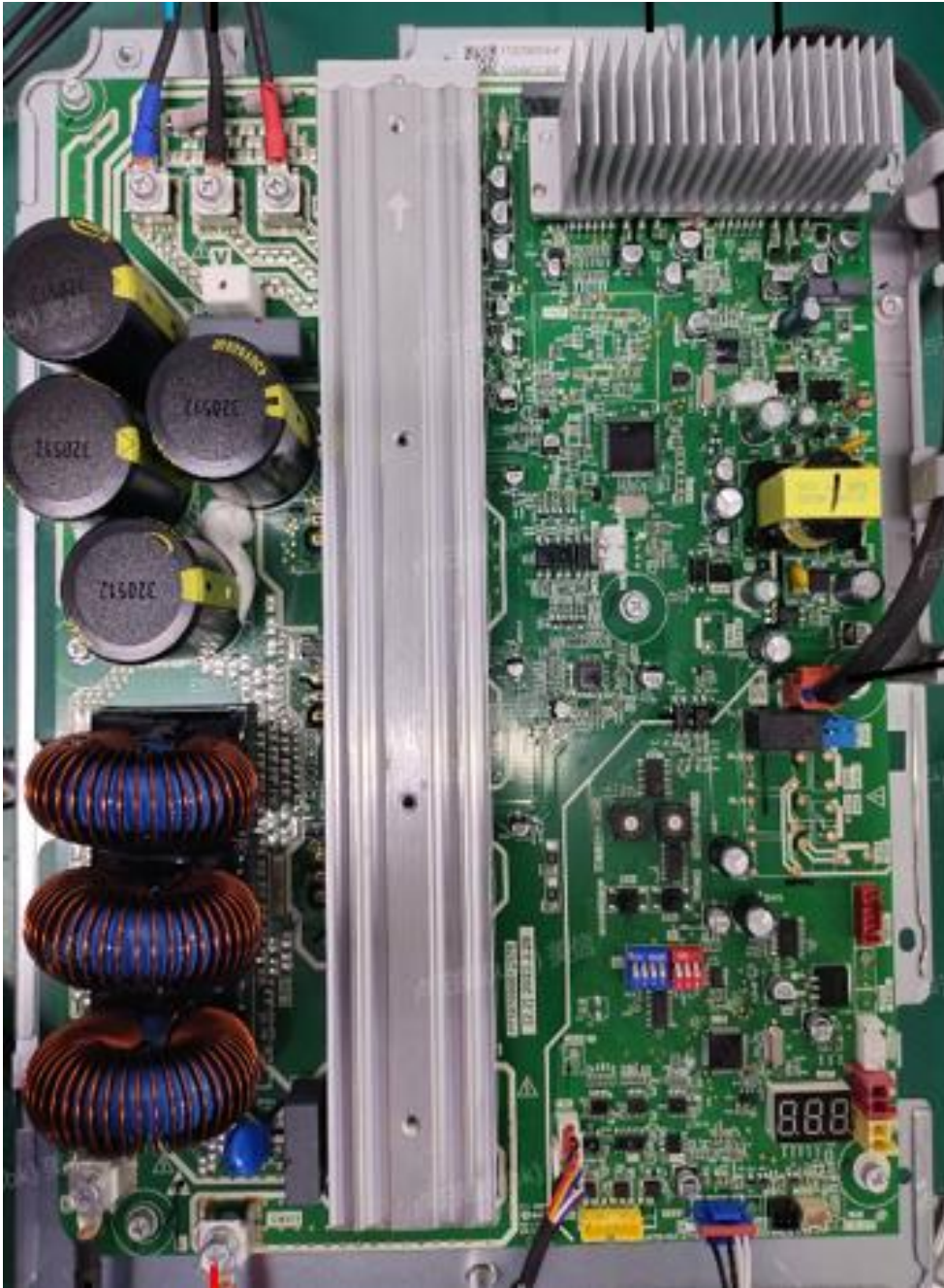
Figure 4-1.1: Electric control box (compressor & fan drive board)
