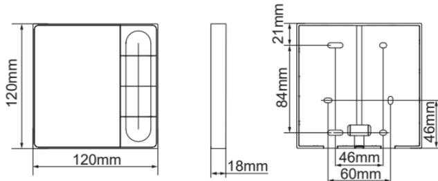
Installation of bottom cap of the wired controller.
