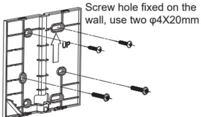
Screw hole installed on 86 electrical box, use two M4X25mm
