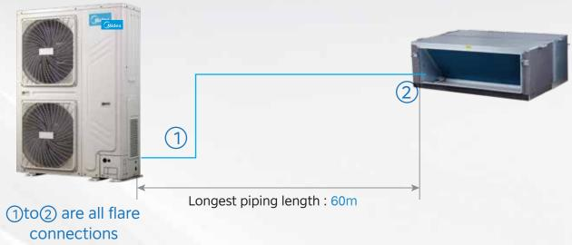
Note: One outdoor unit can only be connected to one indoor unit, and the capacity of the indoor and outdoor units must be the same.
