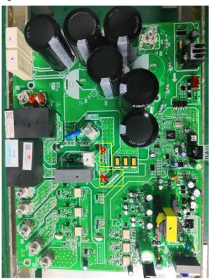
Figure 6-2.1: P and N terminals on Inverter module
