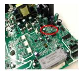
Check the power supply for the compressor inverter module, port CN211 on filter board, the normal voltage should be DC310V; Check the single phase bridge and fuse on filter board; check the connection cable from ODU main PCB port CN4 to filter board port CN8 which is 12V DC power control port.
