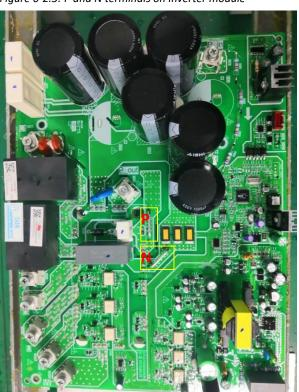
Figure 6-2.3: P and N terminals on Inverter module
