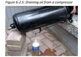
Step 2: Inspect oil from faulty compressor
