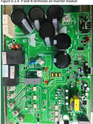
Figure 6-2.4: P and N terminals on Inverter module
