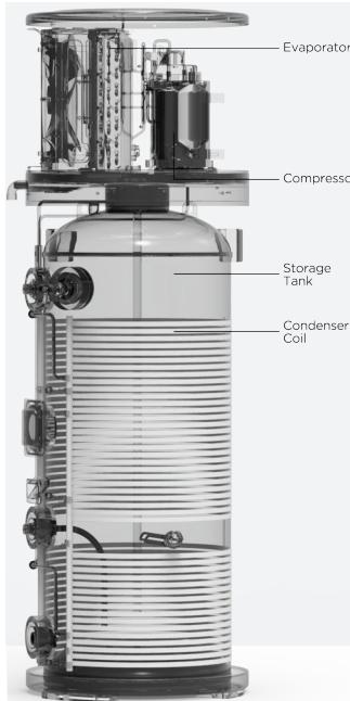
Step 1: A fan draws in air, containing heat energy, across the evaporator. The evaporator turns the liquid refrigerant into a gas.
