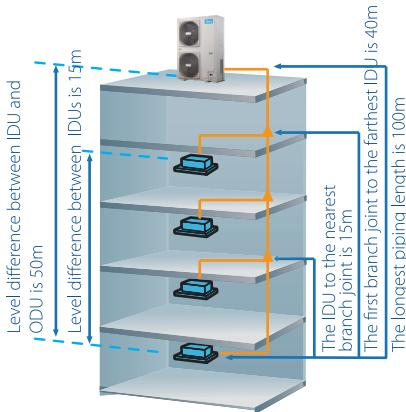
It provides a total piping length possibility of 150m, a maximum height difference between outdoor and indoor units of 50m. The height difference between indoor units can be up to 15m.
