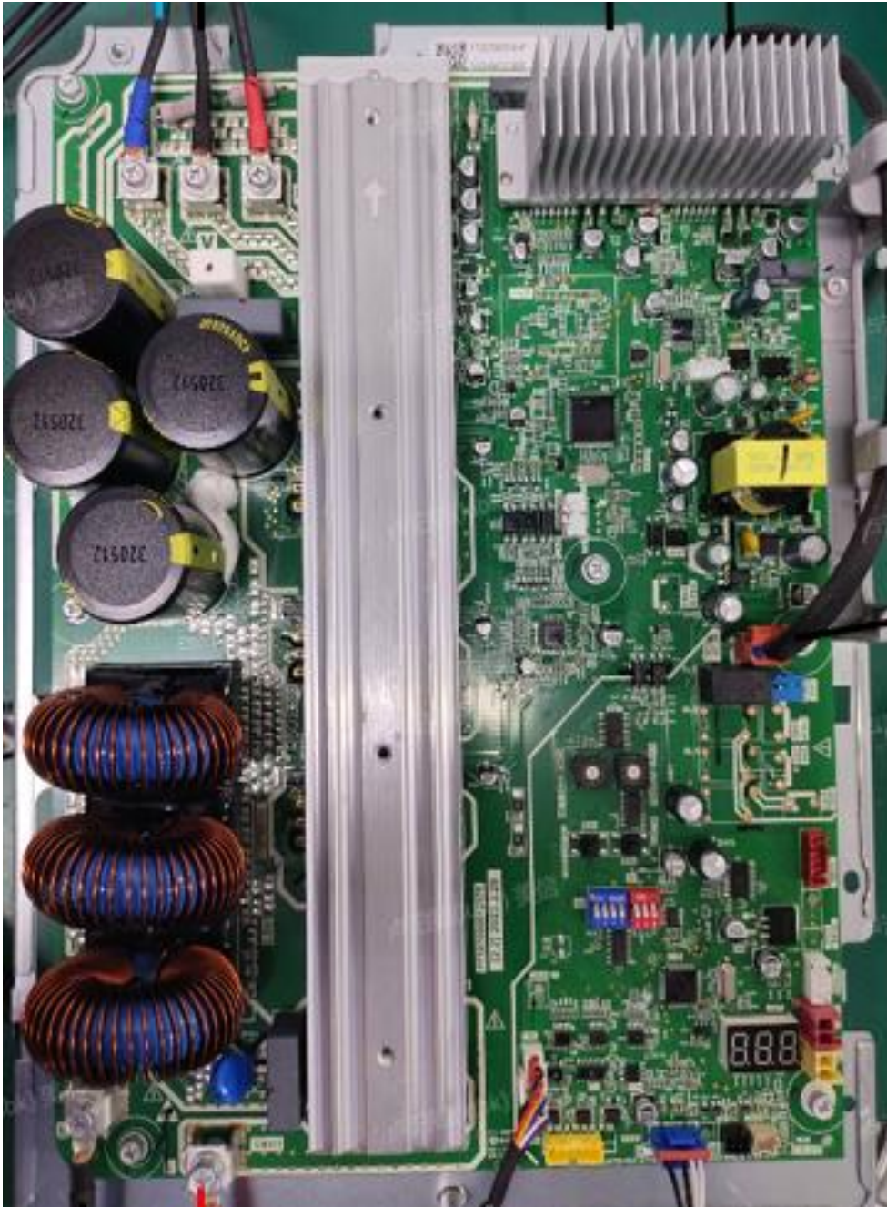
Figure 4-1.1: Electric control box (compressor & fan drive board)
